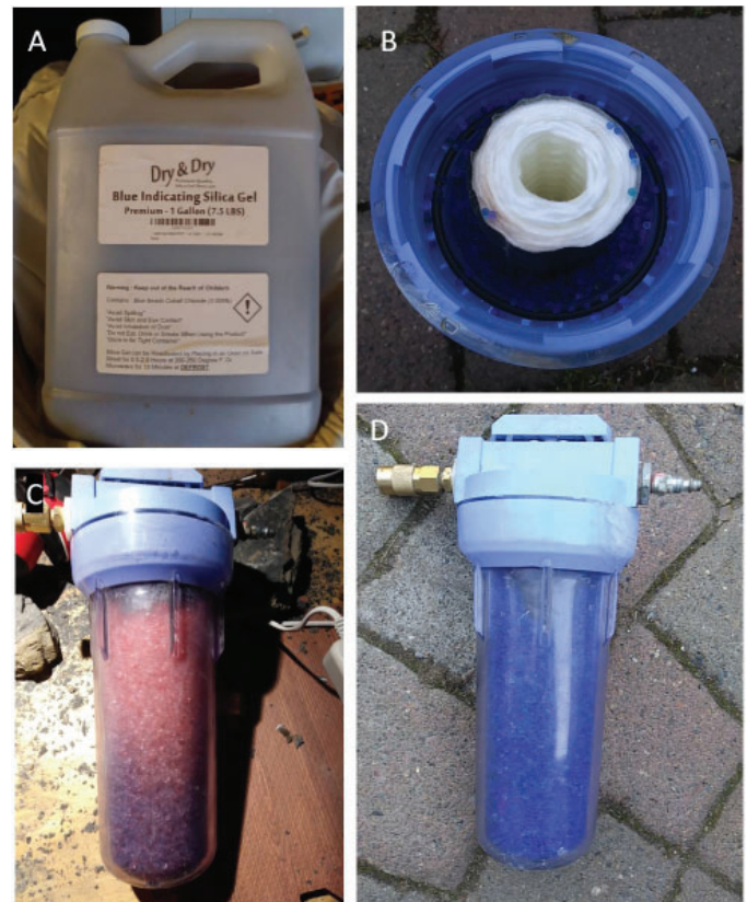
Packaged desiccant (A), loading filter (B), used desiccant (C), fresh desiccant (D).
